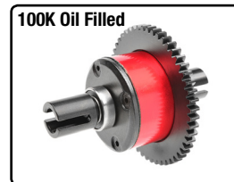
C-00180-685-1 Centre Diff Assembly - Aluminium / Steel - 52T Main Gear - 1 Set
