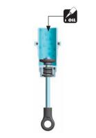
Fill the shock body with shock oil up to the top. Make sure to use same viscosity shock oil as is in the shock.
