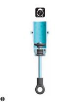
Orient the filled shock vertically for several minutes with the shock shaft fully extended. The remaining air bubbles will release.
