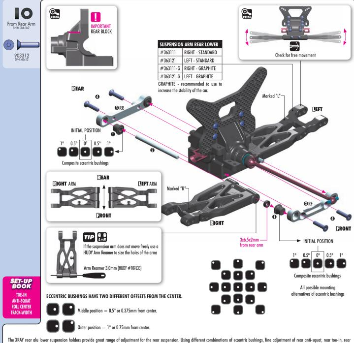
I NE AKAY rear alu lower suspension holders provide great range of adjustment for the rear suspension. Using different combinations of eccentric bushings, tine adjustment of rear anti-squat, rear toe-in, rear roll center, and rear track-width can be obtained. For more information about the influence of rear anti-squat, rear toe-in, rear roll center and rear track width on car handling, please refer to HUDY Set-up Book (#209100).
