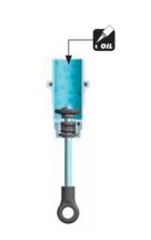
Fill the shock body with shock oil up to the top. Make sure to use same viscosity shock oil as is in the shock.
