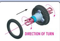
Slide two pulley covers onto the ends of the front axle. Squeeze the covers firmly until they both "snap" over the pulley; it may take a bit of effort to do this.
