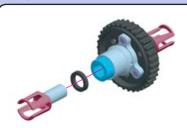
Slide #309319 spacer onto #305131 outdrive shaft.
