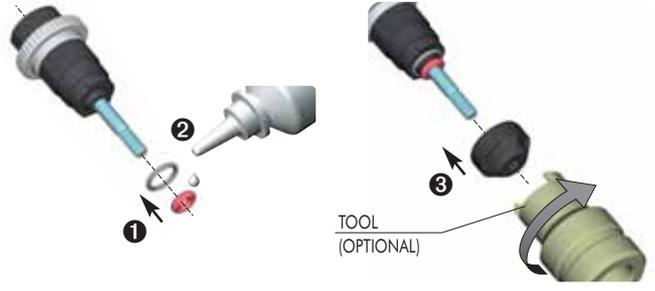
Grip the top of the shock rod's exposed thread with side-cutting pliers. Thread the ball joint onto the shock rod until approximately 1mm of thread is exposed.
