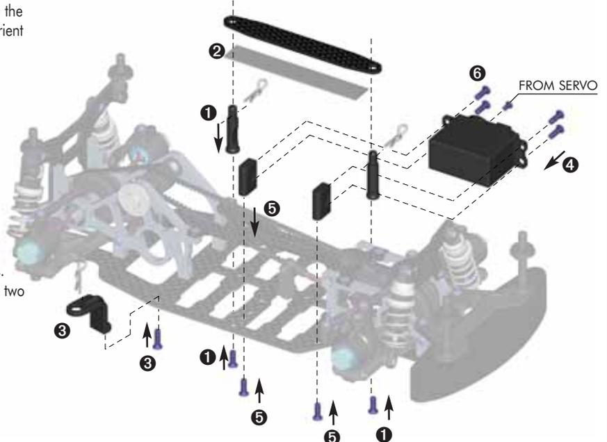
If the servo does not fit properly, you may have to add shims between the servo tabs and the mounting posts.
