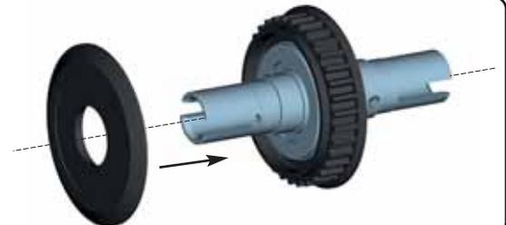
When you need to open the differential, use the shaft of a wrench to spread the dust covers apart to pop them off.
