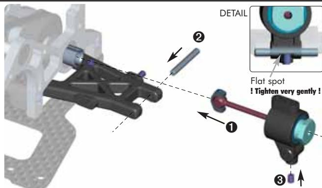
Assemble TWO rear turnbuckles by performing the following steps.
